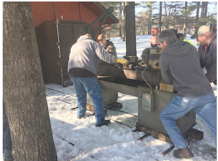
On the Rollers Slowly we rolled the lathe into the depot on the rail heads.
