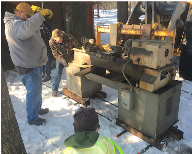
On the Rollers Rob and Marc guide the lathe onto the pipe rollers which were placed on the rails.
