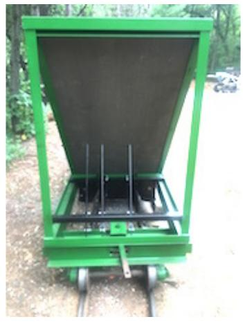
**Controls.** Three levers operate the dumps from the rear of the ballast car. The dump shoots are visible so operators can monitor the flow easily.
