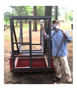
Ballast Car. Marc Brown sprayed the frame of the ballast car. The new car is nearing completion. Soon wee will be spreading ballast with it. Marc's design will permit various methods of placing ballast more directly and with more control.
